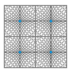
The standard installation is done in a set of 4 pieces. (Figure ①) Install the tiles where the corner with flat surface comes in center, rotating 90° each time. Repeat the standard installation as indicated in Figure ② to complete the installation.
